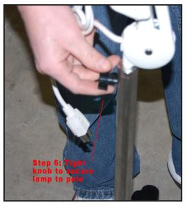
**Step 6**Tighten knob to secure lamp to pole.
